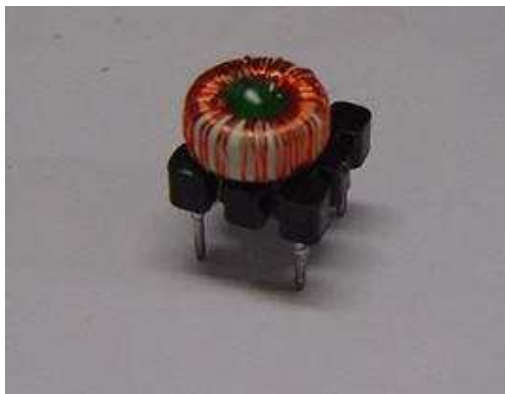
Fig 2 Photograph of MT103 Current Feedback Transformer
